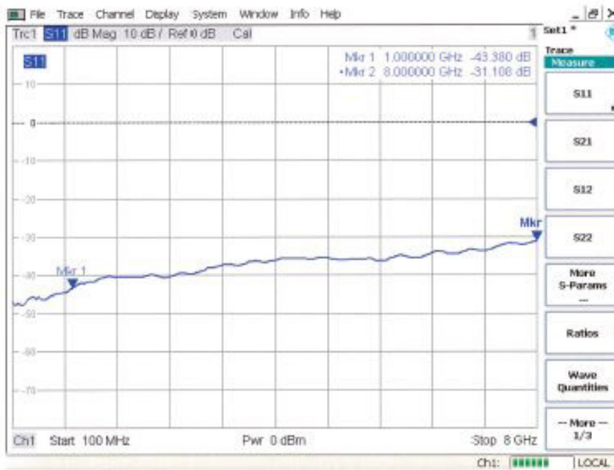
Fig. 4.3.3 Check of the match of a high-performance attenuator pad.
